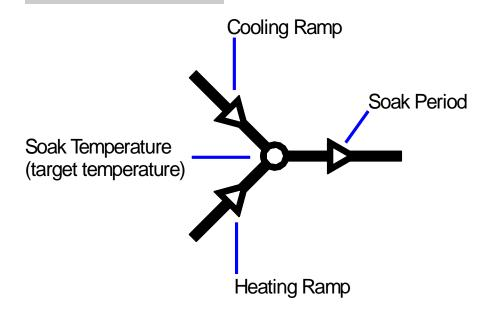
An ST215 firing segment comprises a ramp followed by a soak period. Two segments can be used for simple firing (biscuit firing for example) or several segments can be used per program for complex firing (crystal glazing or glass-making for example).
