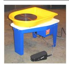
The Bailey Electronic Wheel offers the studio and professional potter a wheel of unparalleled performance and versatility in a compact and user friendly design. The wheel is powered by a super smooth 0.5hp motor that is controlled by a computer enhanced VF drive that due to its unique design can generate up to the peak equivalent of 1hp under heavy loads. This enables the wheel to give constant smooth power throughout the speed range and is extremely quiet in operation.
